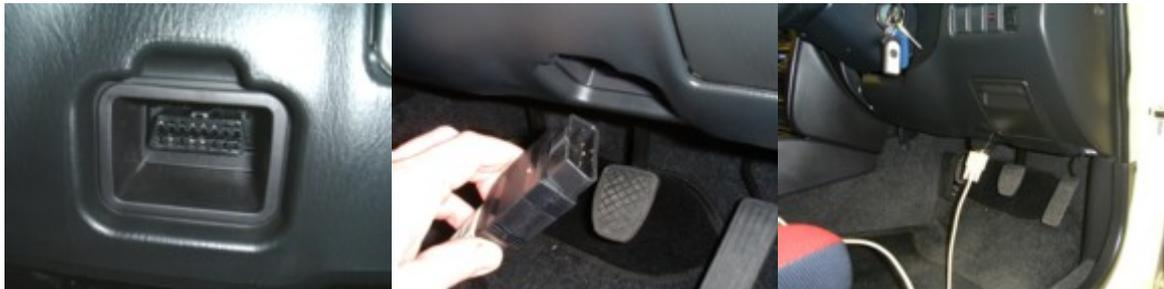
Turn on the ignition switch of the car fully, so that the electrical systems are powered. You are now ready to use DeltaDash with the car.
